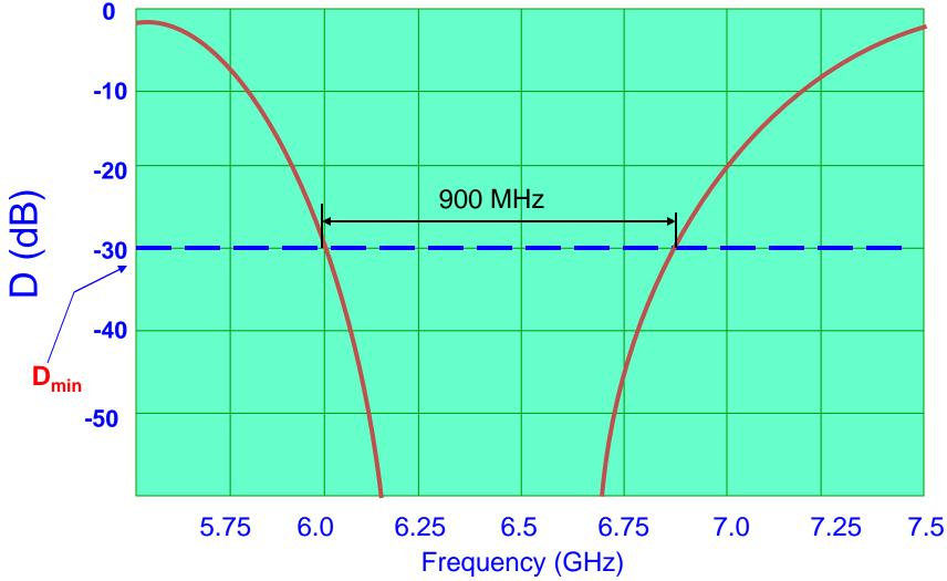
Note that the directivity is better than  $D_{min}$ = -30 dB over a bandwidth of 900 MHz centered about 6.45 GHz.
