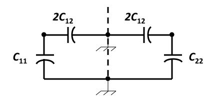
The effective capacitance between either strip conductor and ground is
