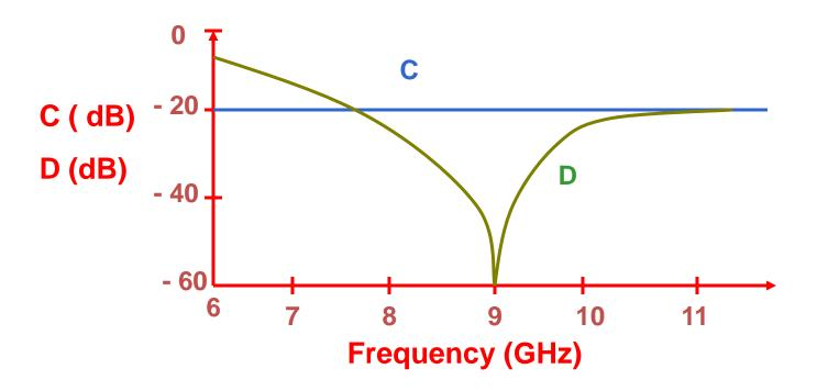
Note: Coupling very broad band, directivity is very narrow band (for single-hole coupler)
