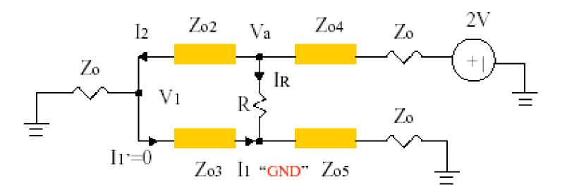
$$\begin{split} V_1 &= j I_1 Z_{o3} \to I_1 = \frac{V_1}{j Z_{o3}} \\ V_a &= j Z_{o2} I_2, I_R = \frac{V_a}{R}, I_R + I_1 = 0 \to R = \frac{Z_{o2} Z_{o3}}{Z_o} = \frac{1 + K^2}{K} Z_o \end{split}$$
