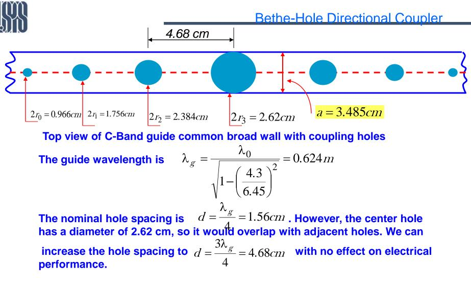
The total length of the common broad wall section with coupling holes is ~ 30 cm, which is fairly large WG section.
