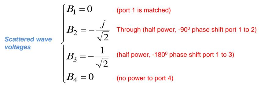
The bandwidth of a single branch-line hybrid is about 10% - 20%, due to the requirement that the top and bottom lines are  $\lambda/4$  in length. We can obtain increased directivity bandwidth (with fairly constant coupling) by using three or more sections.
