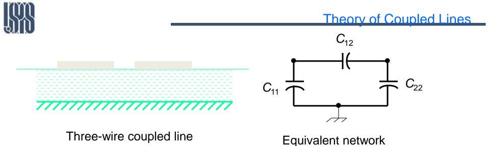
$C_{12} \longrightarrow$  capacitance between two strip conductors in absence of the ground conductor.
