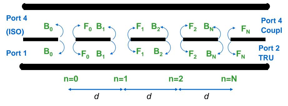
Let a wave of value  $1 \angle 0$  be injected at Port 1. If the holes are small, there is only a small fraction of the power coupled through to the upper guide so that we can assume that the wave amplitude incident on all holes is essentially unity. The hole n causes a scattered wave  $F_n$  to propagate in the forward direction, and another scattered wave  $B_n$  to propagate in the backward direction. Thus the output signals are:
