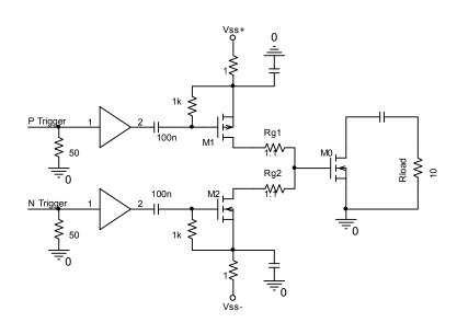
Hybrid schematic: totem pole driver, output MOSFET, and load
