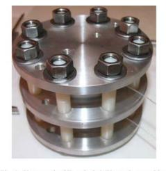
Fig. 4. Photograph of Two-Switch Electrode assembly.
