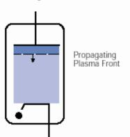
3. Electrons from grid-cathode region create a dense plasma in the grid-anode region. The plasma front propagates toward the cathode via breakdown of gas.
