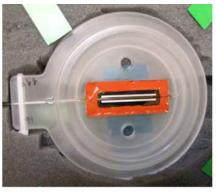
Fig. 3. Photograph of PIMM optical thyristor
