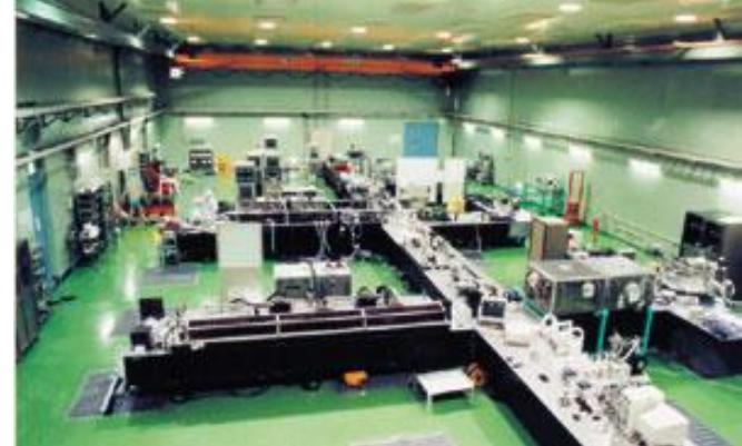
The High Peak Power T 3 Laser 100 TW (1.9J) at JAERI Kansai. Upgrading to 1 PW system. ( a_0 \sim 10 \rightarrow 30 )
