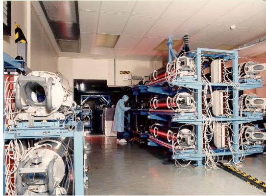
The Vulcan 100 TW (2600 J) Nd:glass system at RAL. Upgrading to 1 PW system. ( a_0 \sim 10 \rightarrow 30 )
