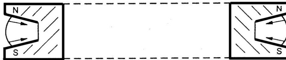
Cross section of weak focusing circular accelerator
