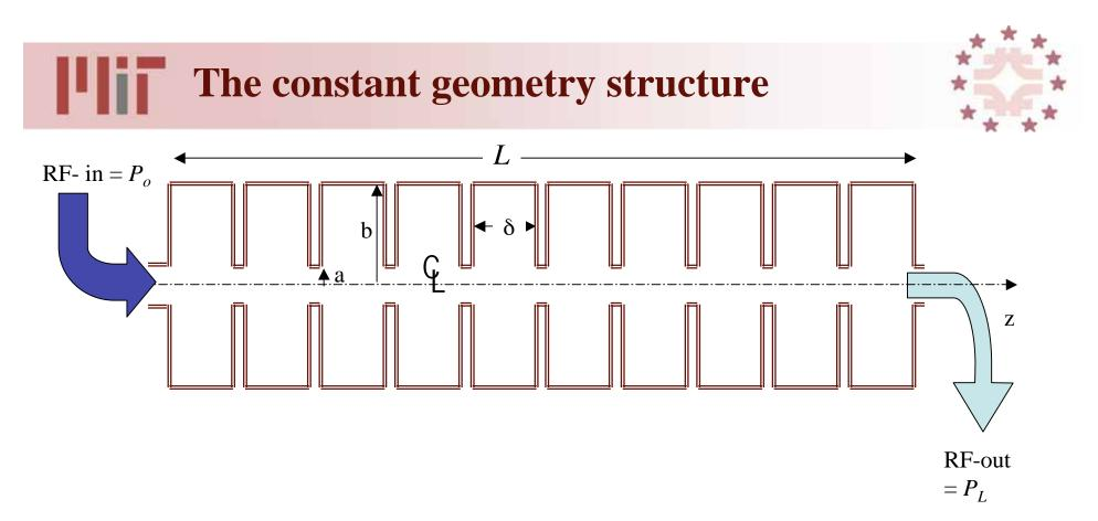
In a structure with a constant geometry, the inductance & capacitance per unit length are constant
