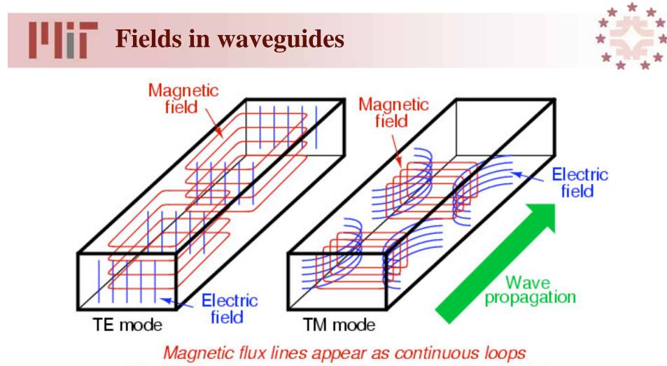
Electric flux lines appear with beginning and end points
