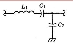
Propagation is cut-off at low frequencies
