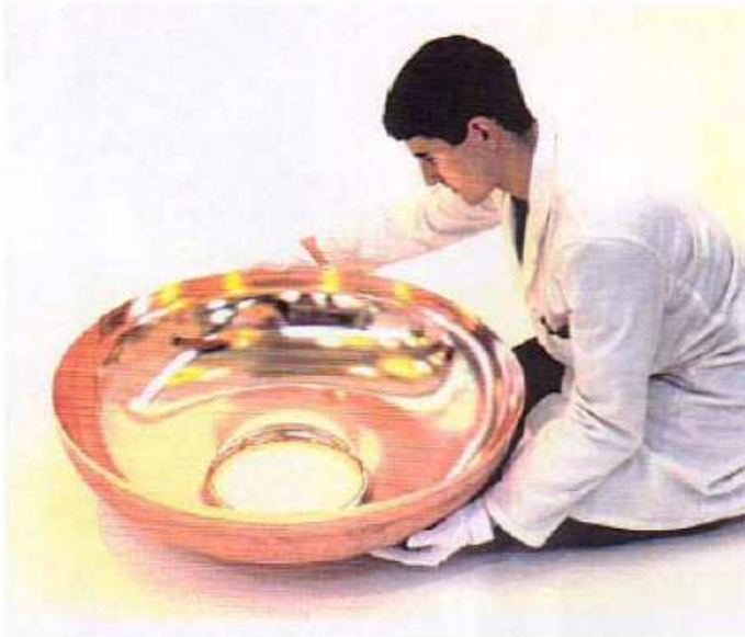
Copper half cell for LEP-II SC cavity
