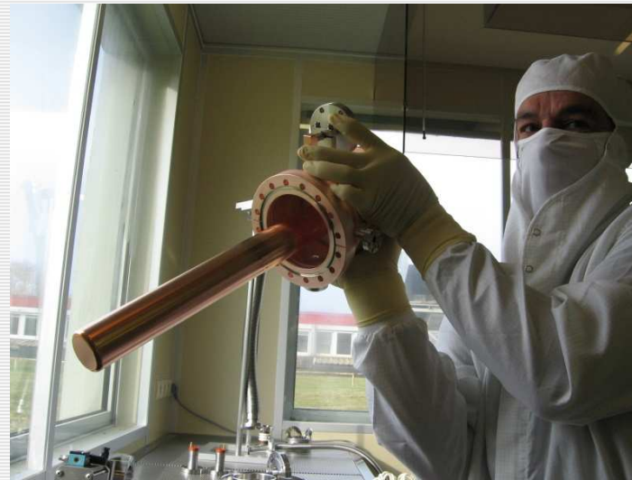
Ceramic disk window with an integrated antenna
