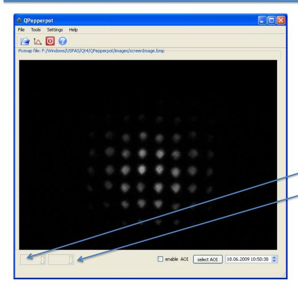
Clicking the left mouse button on the image creates a hor/ver cursor which allows to check the alignment.
