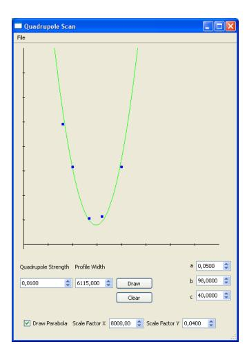
The square of the beam width is Plottet over the "Quadrupole Strength" or 1/f where f is the focal length of the lens
