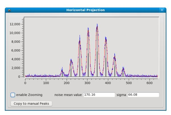
Projection box comes up Through "Tools" menu or histogram button on the tool bar. Blue curve: raw data Red curve: low pass filtered data Black curve: peaks (hole image) Each histogram may be switched on or off from the Tools menu
