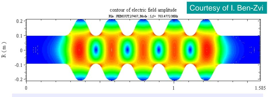
Develop CW SRF cavity for high intensity beams: Large bore, 700 MHz cavity with ferrite HOM dampers and high beam break-up threshold BNL-JLAB collaboration
