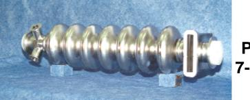
Prototype 7-cell cavity
