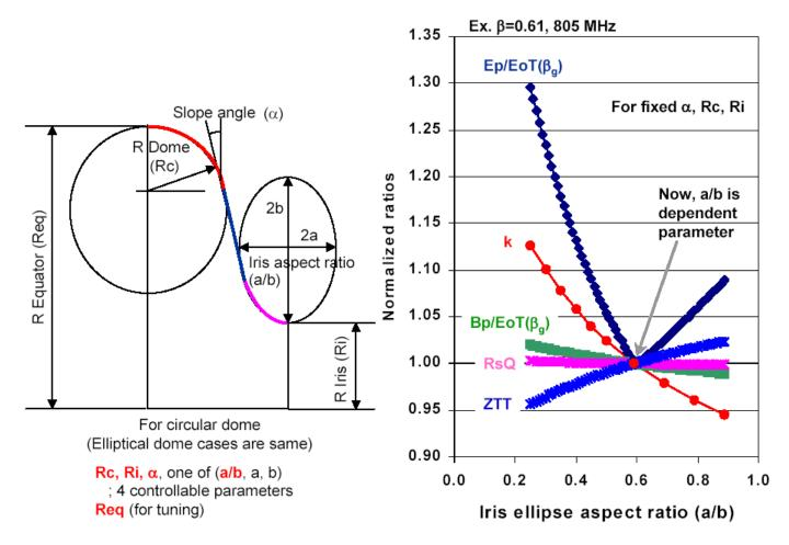
Elliptical cell geometry and dependencies of RF parameters on the ellipse aspect ratio (a/b) at the fixed slope angle, dome radius and bore radius.
