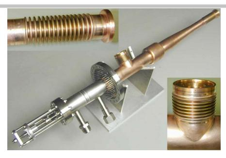
High Power: > 400 kW CW Variable coupling: 2 - 6 E5 High-speed pumping Double window Tested up to 1 MW TW CW 850 kW SW More compact at lower frequencies Allows variability
