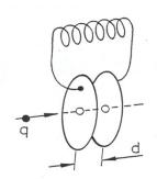
Simple lumped L-C circuit repesenting an accelerating resonator.  $\omega_0^2 = 1/LC$
