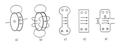
Metamorphosis of the L-C circuit of Fig. 1 into an accelerating cavity (after R.P.Feynman<sup>33)</sup>). Fig. 5d shows the cylindrical "pillbox cavity" and Fig. 5e a slightly modified pillbox cavity with beam holes (typical  $\beta$  between 0.5 and 1.0). Fig. 5c resembles a low  $\beta$  version of the pillbox variety (0.2< $\beta$ <0.5).
