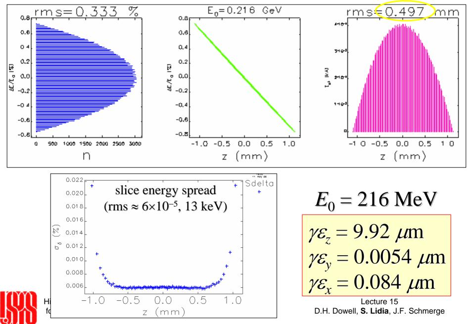
Transverse phase space (left two plots) and longitudinal phase space (right two plots) before (top) and after (bottom) emittance exchange.
