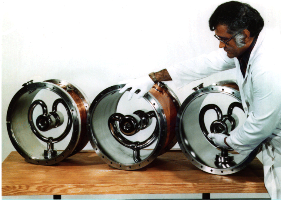
Figure 6. A photograph of the split ring resonators for the ATLAS accelerator for heavy ions (Argonne National Laboratory, Argonne, Illinois, USA [13]). The beam passes through the hole of the two cylinders in the centre (drift tubes). The accelerating field is established between both drift tubes (centre field) and the end plates (not assembled in the photograph) and each drift tube (end fields). The outer housing is made from niobium clad copper to enable cooling by conduction. The inner loop and drift tubes are fabricated from niobium tube and sheet material and are filled with liquid helium for cooling.
