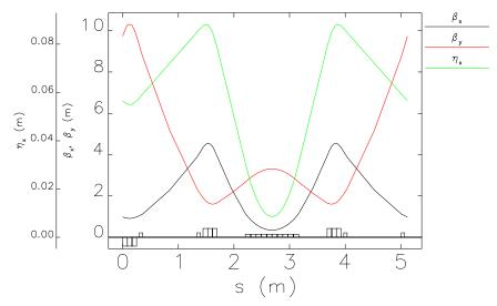
Figure 5.10: TME cell from the NLC damping ring.
