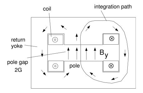
Figure 5.2: Dipole cross section showing integration path.
