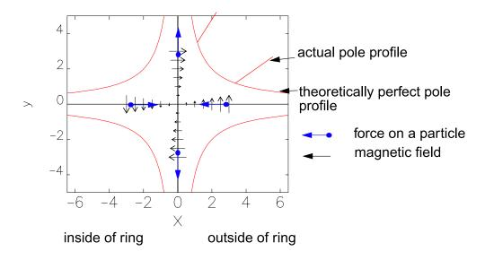
Figure 5.3: Quadrupole cross section showing forces on particles on x- and y-axes.
