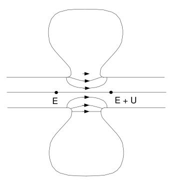
Figure 5.6: Cavity cross section showing the accelerating E-field.
