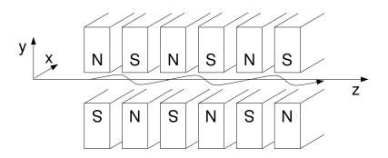
Figure 5.11: Wiggler with undulating trajectory.
