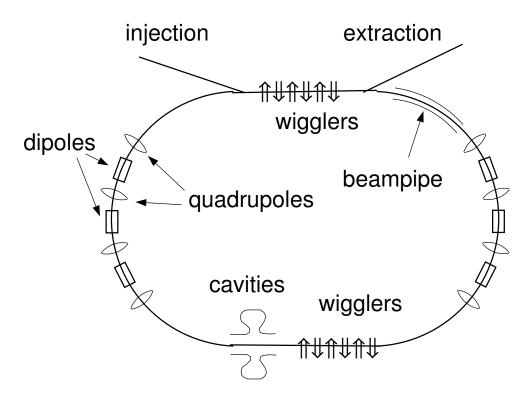
Figure 5.1: Layout of essential damping ring.
