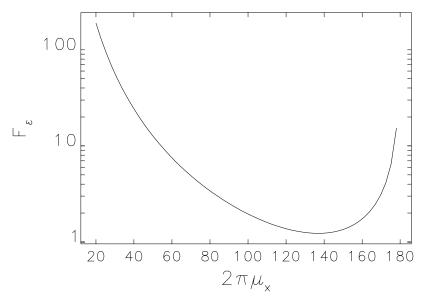
Figure 5.9: Emittance quality factor for FODO cell.
