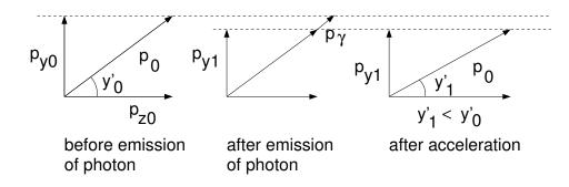
Figure 5.8: Snapshots of particle momentum showing transverse damping.
