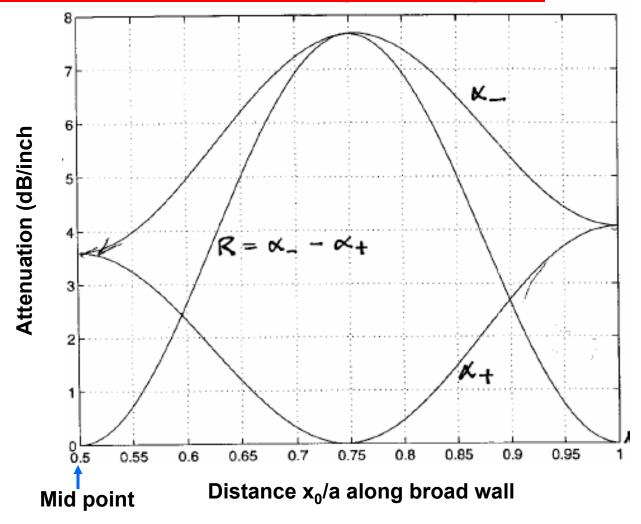
The maximum reverse attenuation  $\alpha_{.}$  is approximately 7.75 dB/inch. Thus the necessary ferrite length is L=25dB/7.75dB/in = 3.23"
