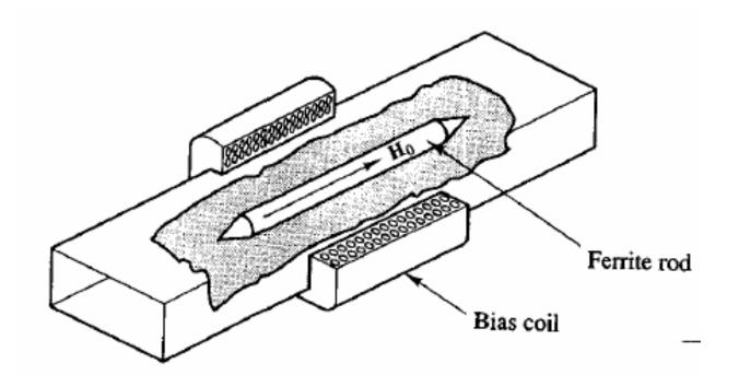
Reciprocal phase shifters are required in scanning antenna phase arrays used in radar or communication systems, where both transmitting and receiving functions are required for any given beam position. The Reggia-spencer phase shifter is such that a reciprocal device. The phase delay through the waveguide is proportional to the d.c. current through the coil, but independent of the direction of the propagation through the guide.
